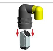
3. Pull float and seal from housing.
