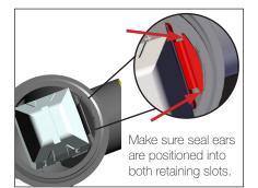
6. Carefully guide seal into slots. Use flathead screwdriver to guide the seal in place.
