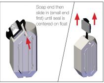
5. Slide in new seal onto float. Pull up on seal to ensure seal is centerted.
